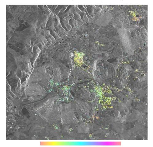
Fig. 3. Linear deformation (temporal baseline 106 days) - one colour cycle stands for 0,02 m (-0,01;0,01)
