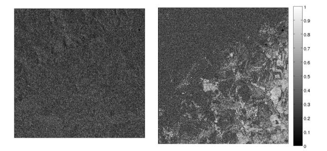
**Fig. 5.** Average coherence of entire images for pairs: 71891-75398 (Jan 2009 – Sep 2009) – 0.18 and 71390-72392 (Dec 2008 – Feb 2009) – 0.29 (maximal coherence)
