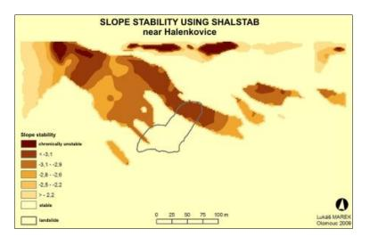
Fig. 2 Stability of slopes near Halenkovice computed in SHALSTAB [9]
