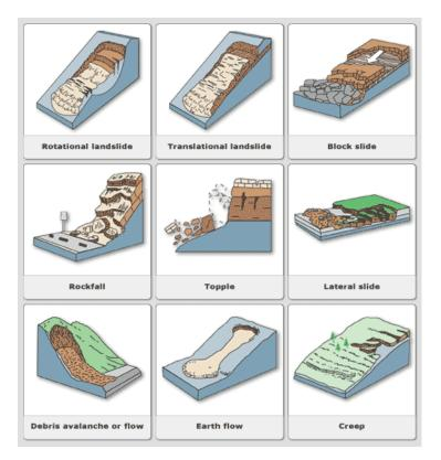
Fig. 1 Possible classification of the slope movements [13]
