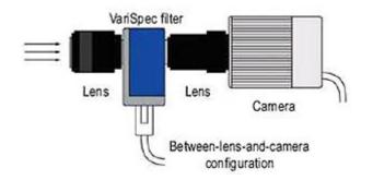
Fig. 4. Configuration of the hyperspectral set: camera, filter and lens
