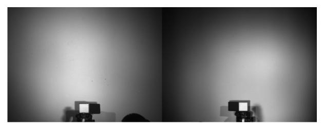
Fig. 7. The effects of vignetting on images acquired using f/4 (left) and f/8 (right) aperture settings.
