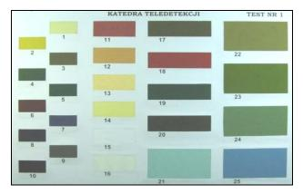
Fig. 5. Test board consisting of a number of different textiles on a white background
