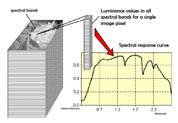
Fig. 2. Acquisition of spectral response curves using a hyperspectral method [5]
