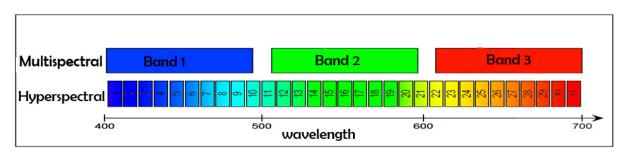
Fig. 3. A comparison of multispectral and hyperspectral bands
