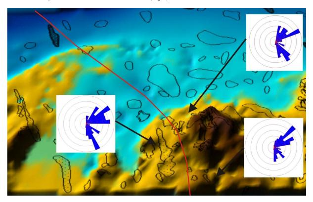
Fig. 3. Relief map of Kolva megaswell with East Kolva fault and lineament rose-diagrams.
