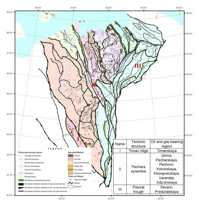
Fig. 1. Map of tectonic and petrogeological zoning with hydrocarbon deposits and local structures.
