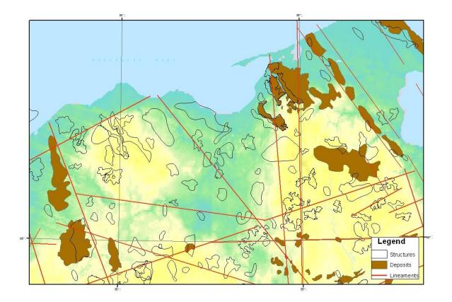
Fig. 2. Map of lengthy lineaments with hydrocarbon deposits and local structures.
