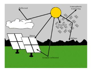
Fig. 1 The sum of the direct (beam), diffuse, and ground-reflected irradiance arriving at the surface is called global irradiance. This can be horizontal or tilted, depending on the surface. Source: NREL
